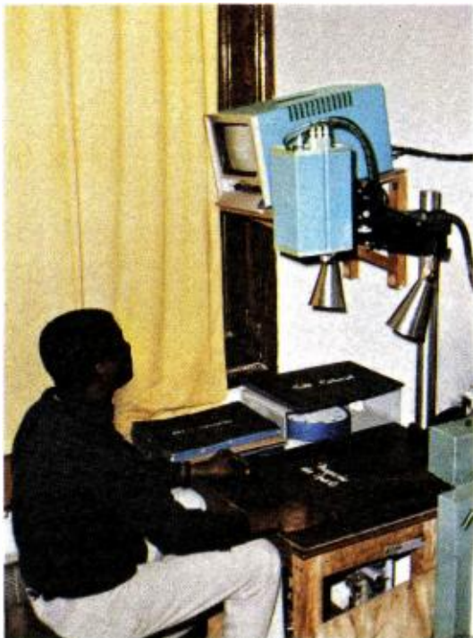
FIG. 8 PK-301 camera as caption scanner for ID's and time announcements.
