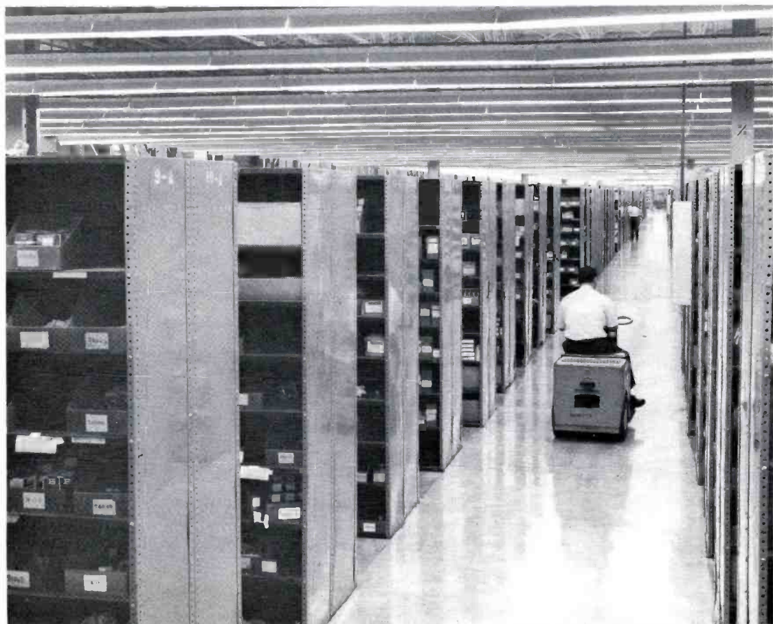
FIG. 5 All the replacement parts are stored in many aisles of bins, row after row, to expedite the shipment of customer orders. Motorized carts are used to get around the huge warehouse.
