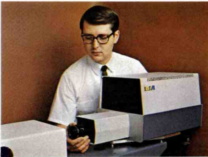
FIG. 4 New 3-vidicon solid-state color film camera, Type PK-610. It may be used on many different film systems. Selling price is $14,750.
