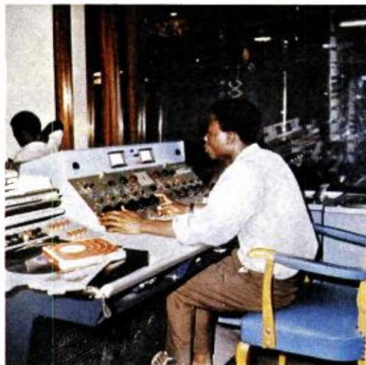
FIG. 6 BC-7A Consolette uses stereo channel for standby.
