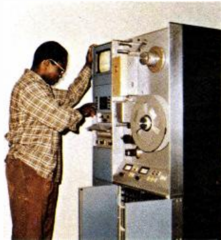
FIG. 9 Tape facilities include remotely controlled TR-4 Tape Recorder and TR-5 Mobile Tape Recorder.
