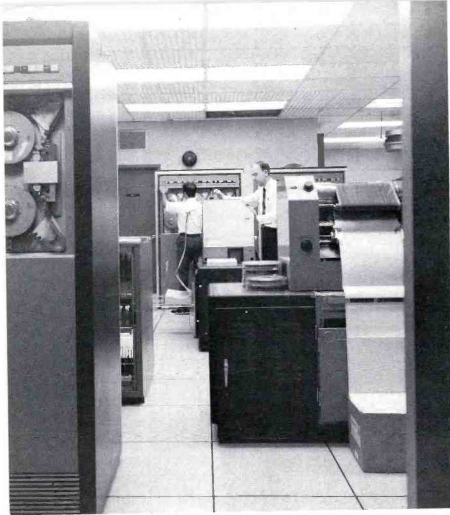
FIG. 2 Two RCA 301 Computer Systems give answers to complex requirements in minutes that would otherwise take months. This highly sophisticated computer system writes at 1200 lines per minute to maintain parts inventories.
